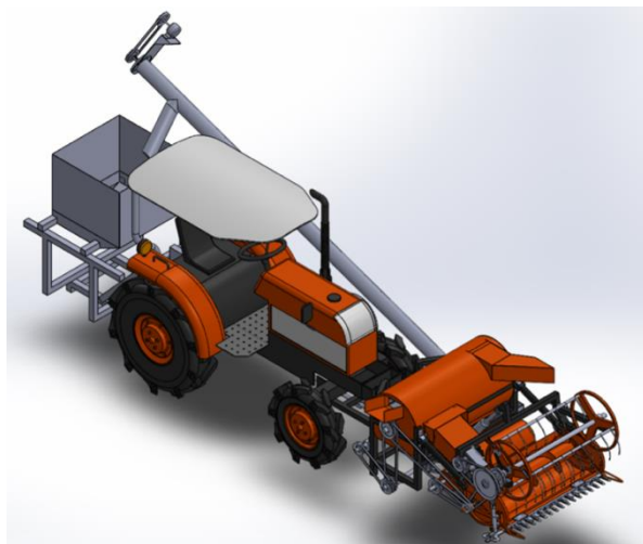
Figure 1 Model of an Upland Rice Combine Harvester Attachment for a Small Tractor (14 hp)
