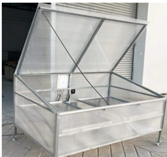
Figure 1 Solar dryer combined with electric heater
