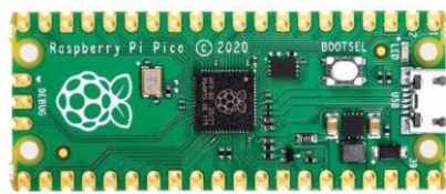
Figure 2 The Raspberry Pi Pico microcontroller board
